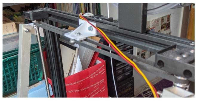
The above picture shows it. There are 20T GT2 cogged wheels (2mm pitch, 6mm wide, 8mm shaft), linked with a 760mm belt. There is a tensioner of my own (FreeCAD) design in the middle, using a couple of 6m wide belt idlers, 3mm shaft diameter.
