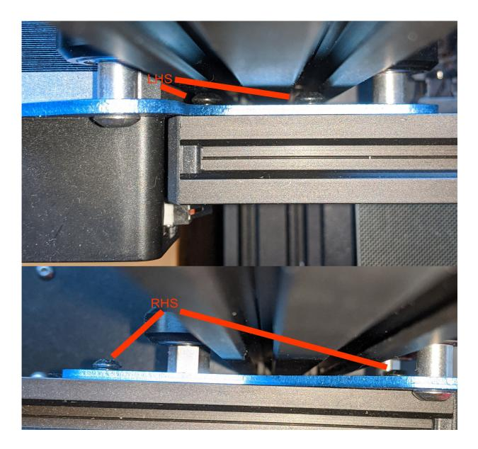
The X runner is firmly screwed to these brackets, it is not a hinge.
